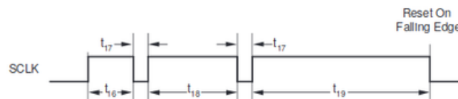
Figure 12. Resetting the DAC1220
